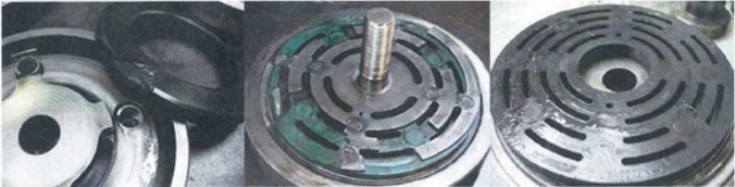
Plate damage caused by sticktion.
