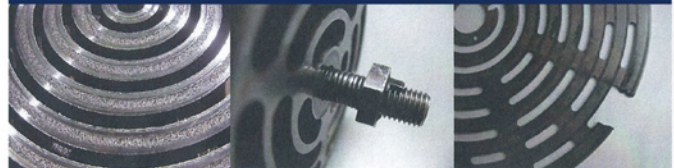
Seat is past retirement thickness.
