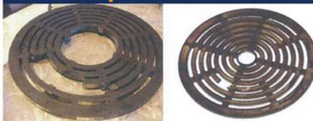
Damaged plates caused by liquid going through the valve.
