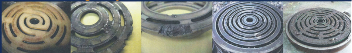
Debris imbedded on sealing plate.
