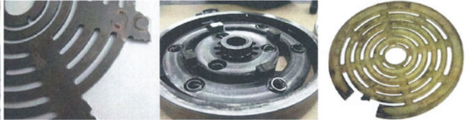
Severe plate failure.
